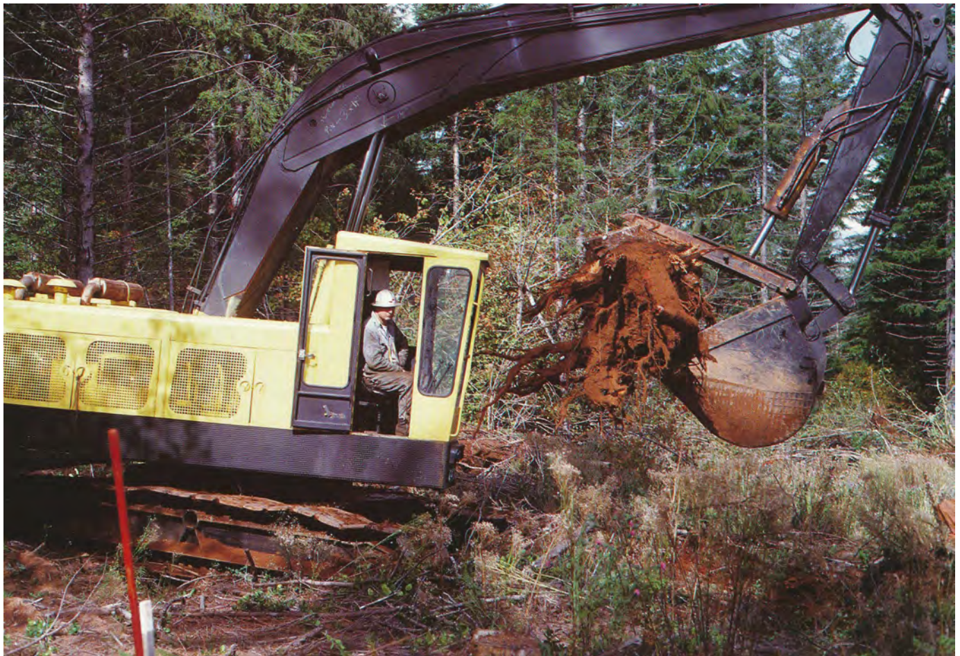
Figure 25—A large excavator with a standard bucket and an optional gripping thumb can be used effectively for stump removal.
